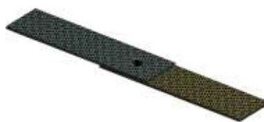
Fig. 2 Meshing of Spot Weld Specimen
