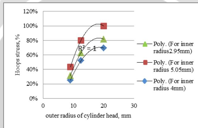
Fig. 10(b) Effect of outer radius 1)9 2) 12.5 3) 20mm on hoops stress when inner radius of cylinder head is 2.95mm, 5.05mm and 4mm respectively
