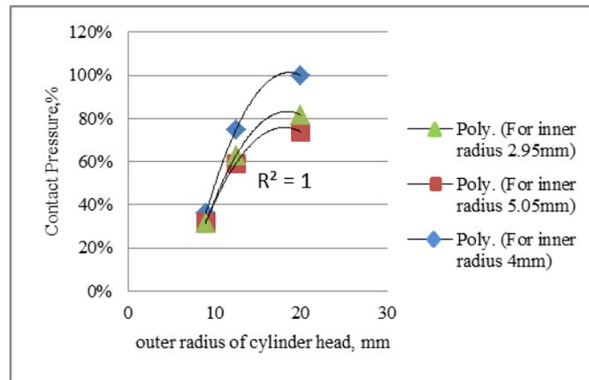
Fig. 10(a) Effect of outer radius 1)9 2) 12.5 3) 20mm on contact pressure when inner radius of cylinder head is 2.95mm, 5.05mm and 4mm respectively
