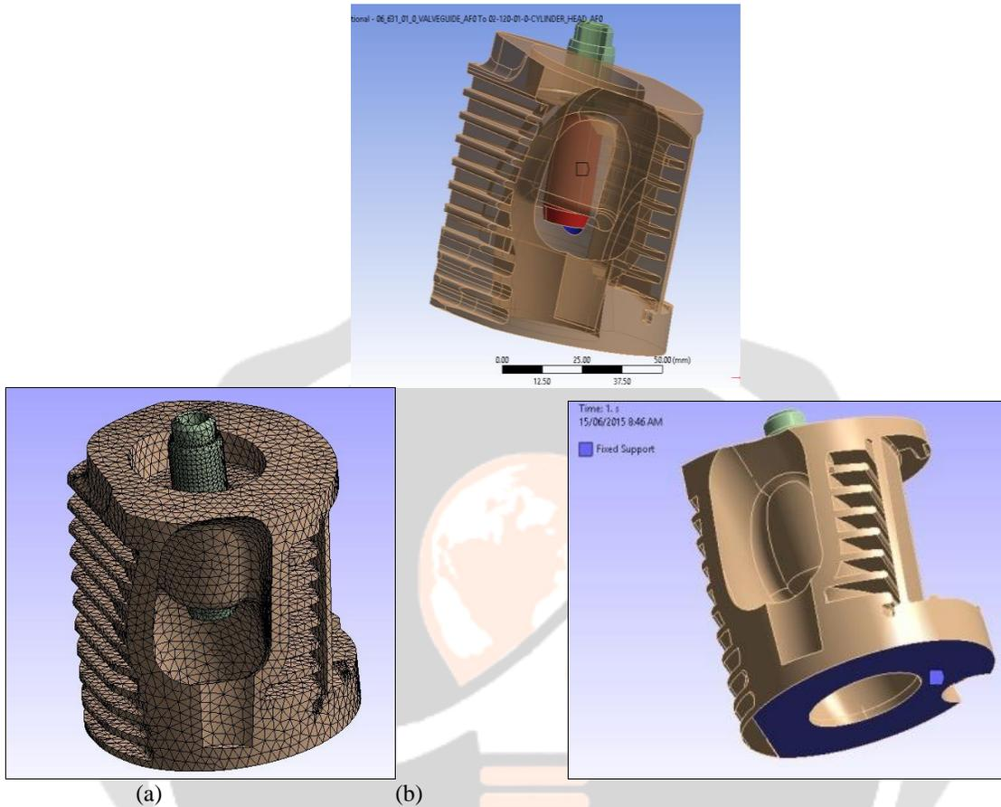
Fig. 2 Cylinder head and valve guide assembly a) Contact Finite element mesh b) Fixed support
