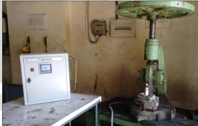
Fig.5 Experimental setup for calculating Push out force
