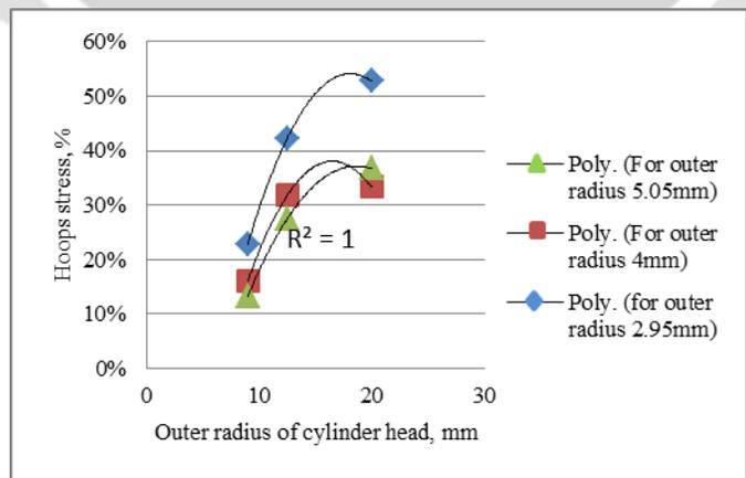
Fig. 8(b) Effect of outer radius 1) 9 2) 12.5 3) 20mm on hoops stress when inner radius of cylinder head is 5.05mm, 4mm and 2.95mm respectively
