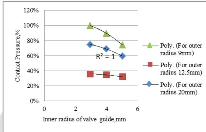
Fig. 9(a) Effect of inner radius 1)2.65 2) 4 3) 5.05mm on contact pressure when outer radius of cylinder head is 9mm, 12.5mm and 20mm respectively
