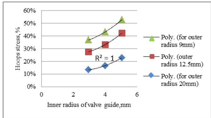
Fig. 6(b) Effect of inner radius 1) 2.65 2) 4 3) 5.05mm on hoops stress when outer radius of cylinder head is 9mm, 12.5mm and 20mm respectively
