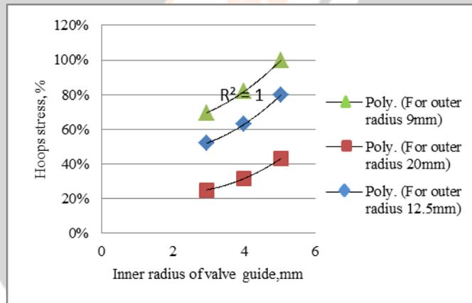
Fig. 9(b) Effect of inner radius 1)2.65 2) 4 3) 5.05mm on hoops stress when outer radius of cylinder head is 9mm, 20mm and 12.5mm respectively
