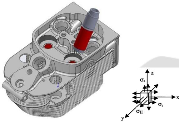
Fig. 1 a. Actual cylinder head and valve guide assembly
