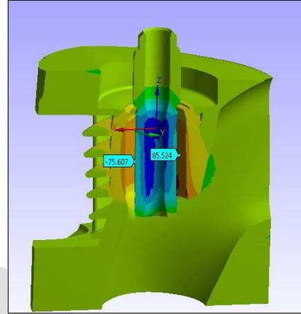
Fig. 4 hoops stress at valve guide and cylinder head
