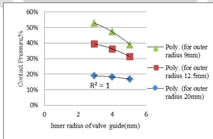
Fig. 6(a) Effect of inner radius 1)2.65 2) 4 3) 5.05mm on contact pressure when outer radius of cylinder head is 9mm, 12.5mm and 20mm respectively
