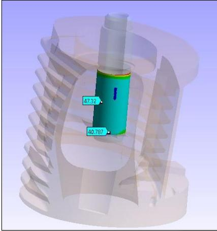
Fig. 3 Contact pressure in cylinder head and valve guide assembly
