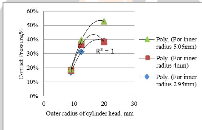
Fig. 8(a) Effect of outer radius 1) 9 2) 12.5 3) 20mm on contact pressure when inner radius of cylinder head is 5.05mm, 4mm and 2.95mm respectively
