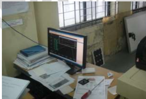
Fig.4 I-V characteristics measurement for solar module under Bangladeshi climatic condition
