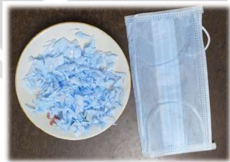
Fig.3 Face Mask [Non-Woven Geotextile Material]
