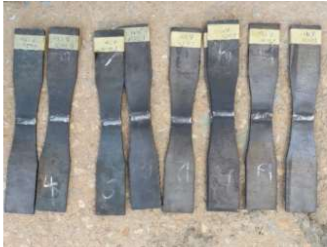
Figure (1) specimens welded using SMAW process
