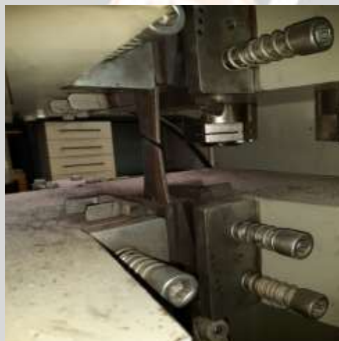
Figure (2) low carbon Steel specimen tested without welding.
