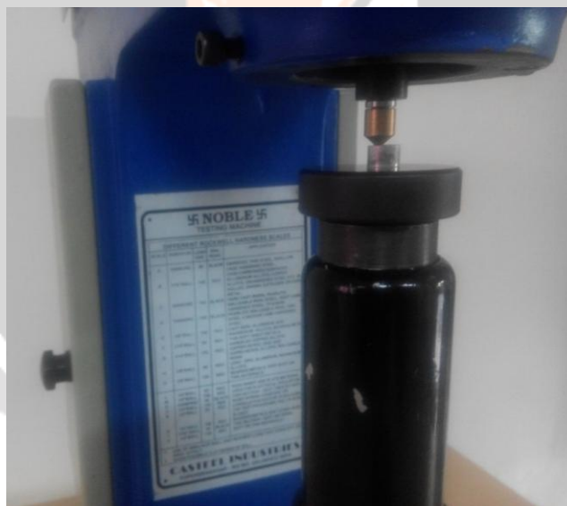
Fig. 14- Sample under indenter for Brinell hardness test
