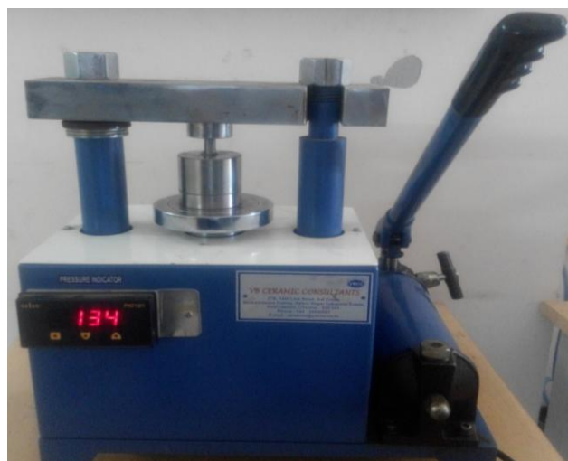
Fig 5- Pneumatic compaction machine
