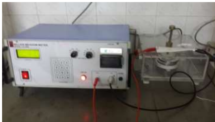
Fig -3: Equipments used to measure electrical insulation
