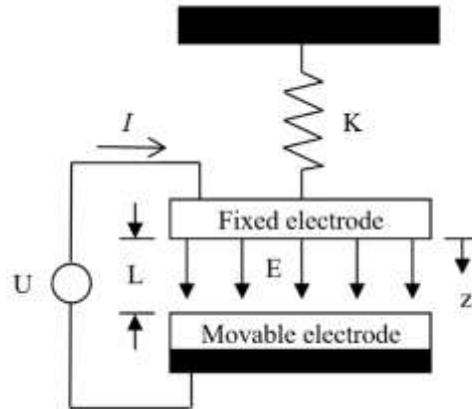
**Fig -2:** FP optical filter model in the form of two parallel electrodes
