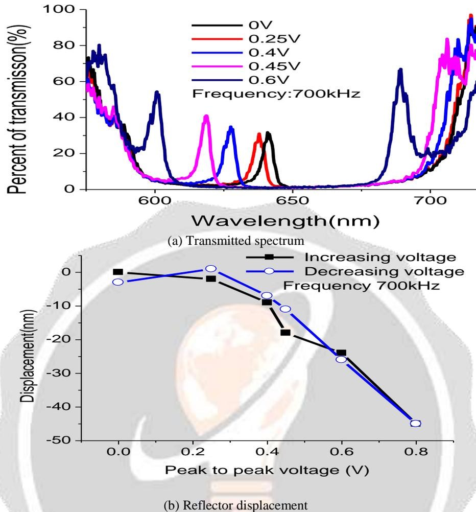
**Fig -4:** Control at 700KHz frequency
