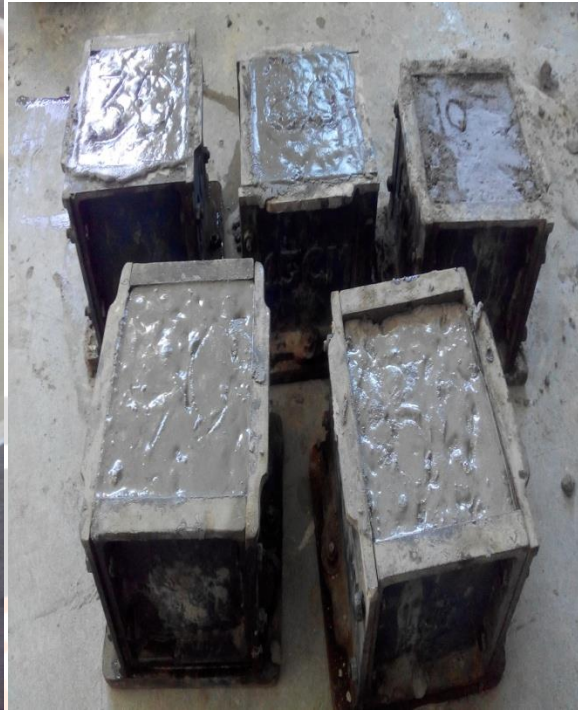
Casting of cubes
