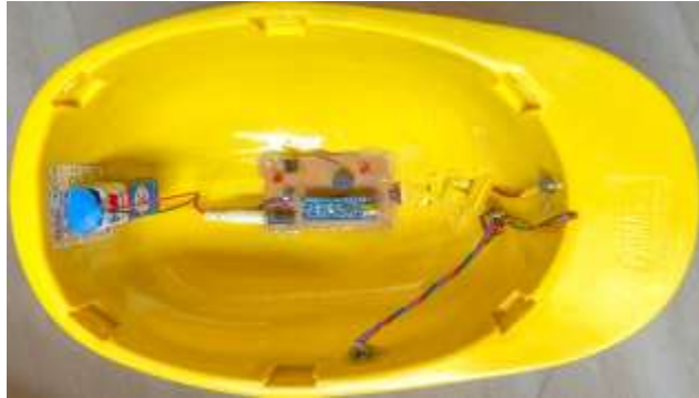
Fig 3. Circuit Connection (Inside)
