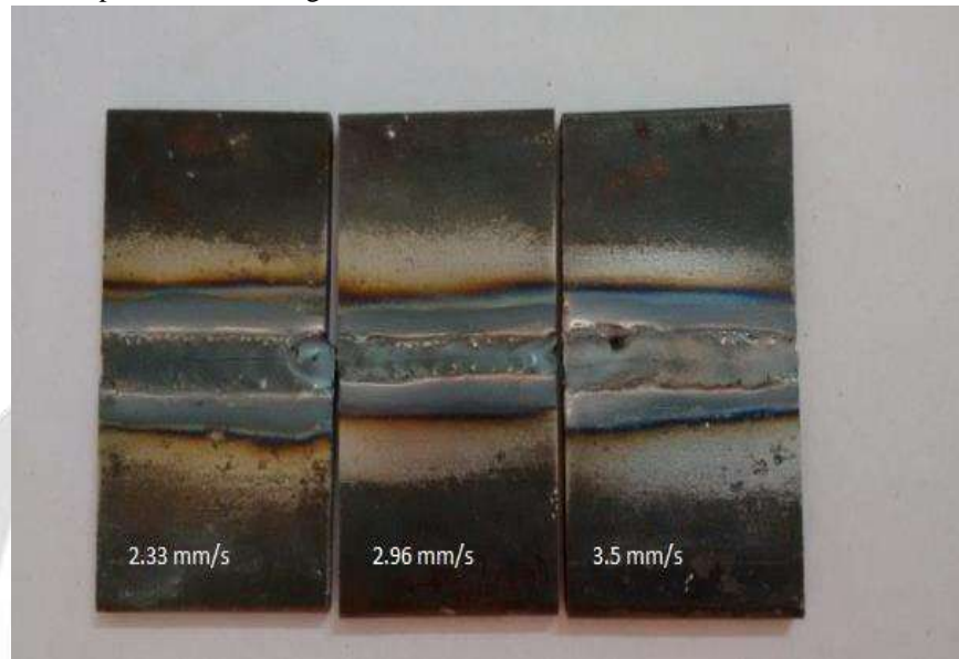
Fig. 2 TIG welded specimen with TiO 2 flux at 210 A current
