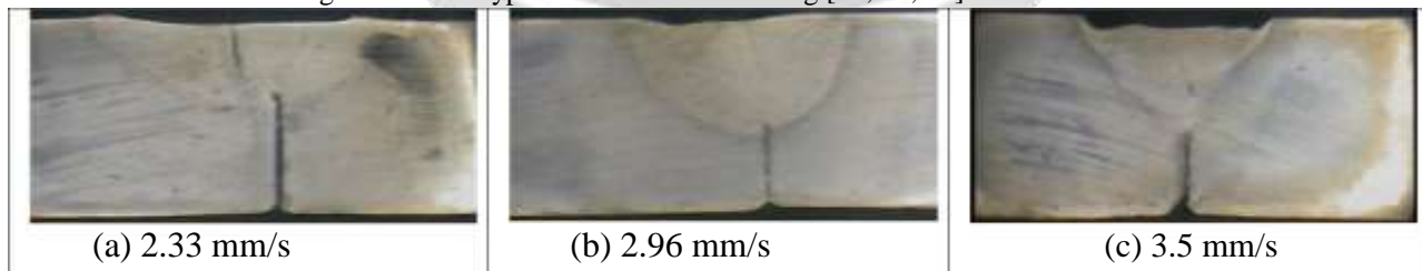
Fig. 3 Optical microscopic Image at weld zone of TIG welded specimen with use of TiO 2 flux
