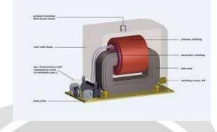
Voltage transformers (VT), also called potential transformers (PT), are a parallel connected type of instrument transformer. They are designed to present negligible load to the supply being measured and have an accurate voltage ratio and phase relationship to enable accurate secondary connected metering.
