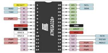
The Atmega328 is a very popular microcontroller chip produced by Atmel. It is an 8-bit microcontroller that has 32K of flash memory, 1K of EEPROM, and 2K of internal SRAM.
