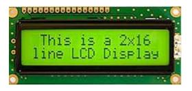
LCD (Liquid Crystal Display) screen is an electronic display module and find a wide range of applications. A 16x2 LCD display is very basic module and is very commonly used in various devices and circuits. These modules are preferred over seven segments and other multi segment LEDs.
