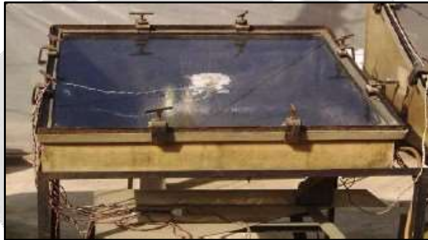
Fig -3 Photograph of the experimental single sloped solar still (Fronting due South) [4]
