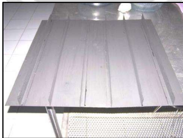
Fig -12 Strip-fins attached on Absorber Plate [14]
