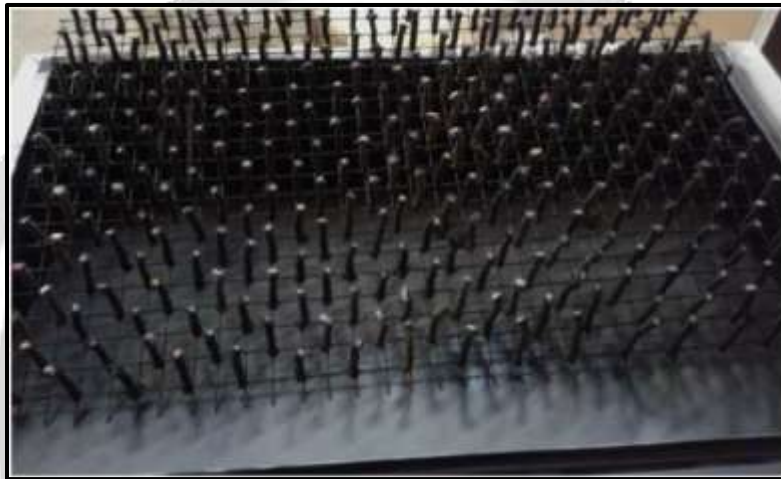
Fig -16 Pin fin of wick elements placed on the absorber plate of solar still [12]
