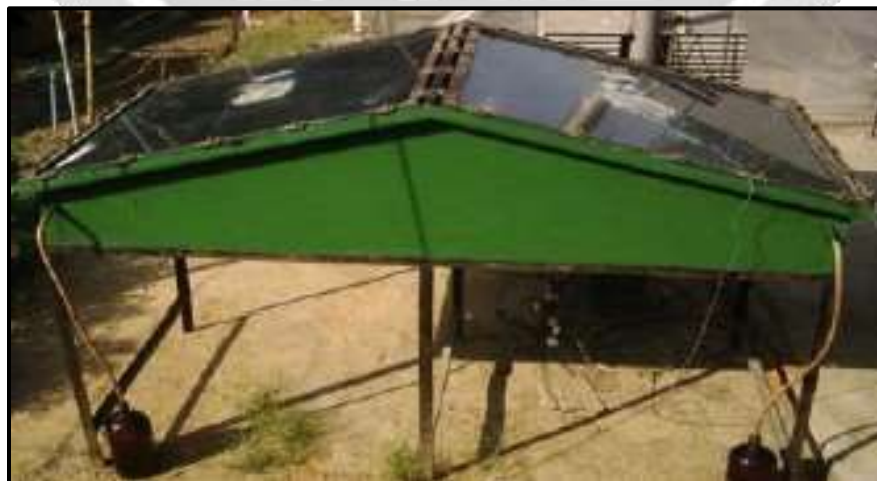
Fig -4 Photograph of the experimental double sloped solar still (Slopes fronting due East - West) [4]
