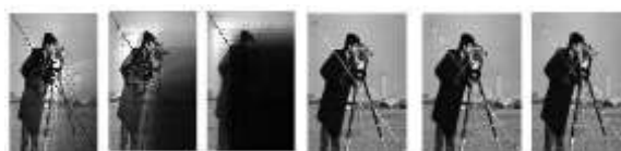
Fig. 6. a)-c) Shows the extracted watermark after JPEG compression. d)-f) Shows the extracted watermark after noising attack.
