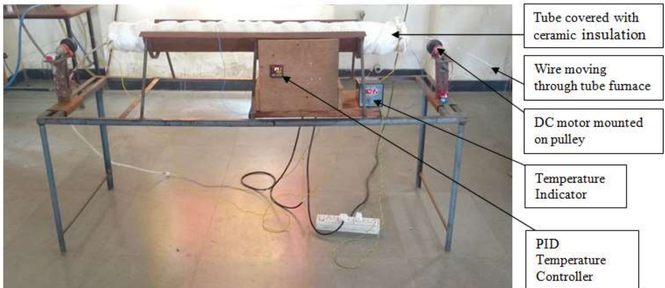
Fig. 7 The actual setup of developed Unsteady State Continuous Annealing Furnace [8]
