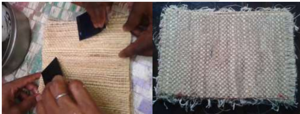
Fig: 3.2 Hand Lay-up method
