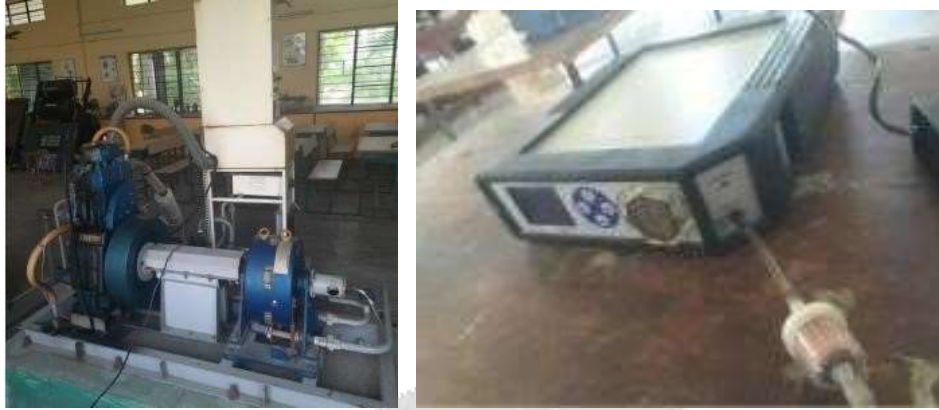
Fig:4. (a) AVL DI GAS 444 Exhaust gas Analyzers (EGA) form assuring emission gases (b) Inlet exhaust gas from the engine to EGA
