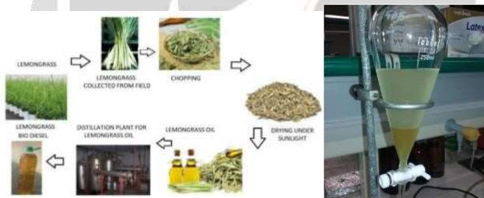
Fig:2. Extraction and trans-esterification of Lemon grass oil
