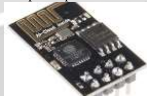
Fig 5:- ESP8266 (Wi-Fi-Cloud module)
