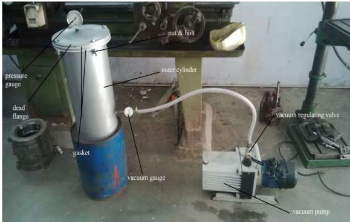
Figure 3: Experimental Setup of LN 2 Tank
