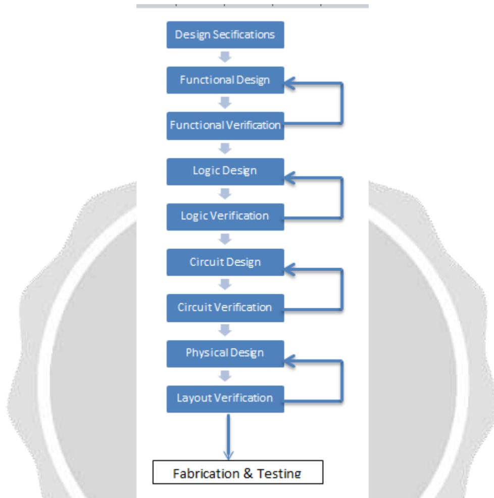
The design flow starts from the specifications gained by the user/clients. As per the specification like technology node, Chip density, Area, Power, Timing etc, process of designing the standard cells started. The flow is then divided into 6 modules:
