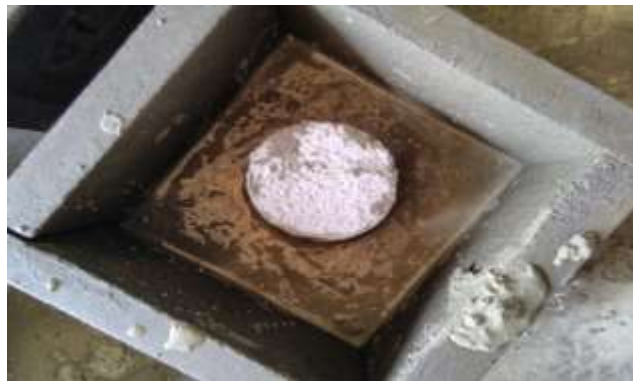
Fig 4: Placing of Specimen in Concrete Cube
