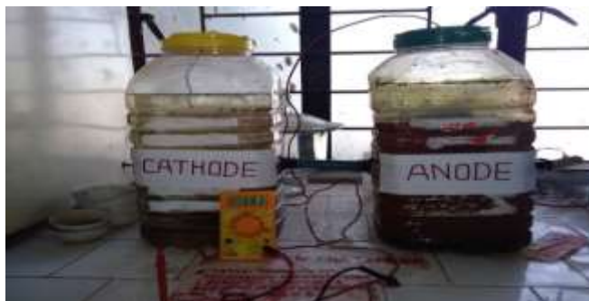
Fig. 2 Double chambered MFC
