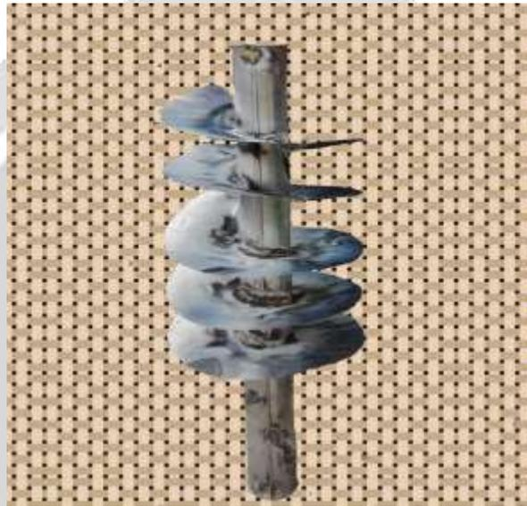
**Figure 1:** Archimedes turbine
