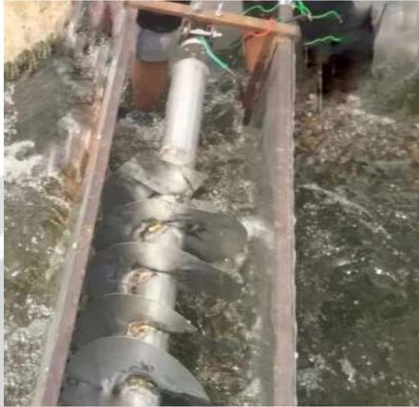
**Figure 2:** installation of ultra power generator with Archimedes screw
