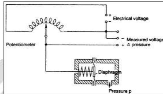
**Fig. 3.1** Deflection as a direct indication of pressure.
