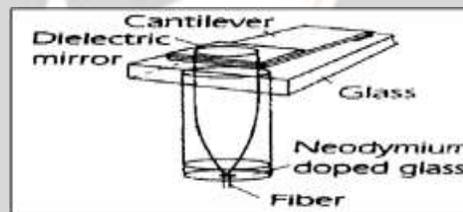
**Fig. 9.1** Cantilever-type acceleration sensors.
