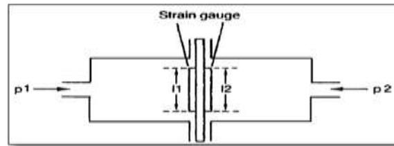
**Fig. 3.3** Strain gauge for measurement of pressure.
