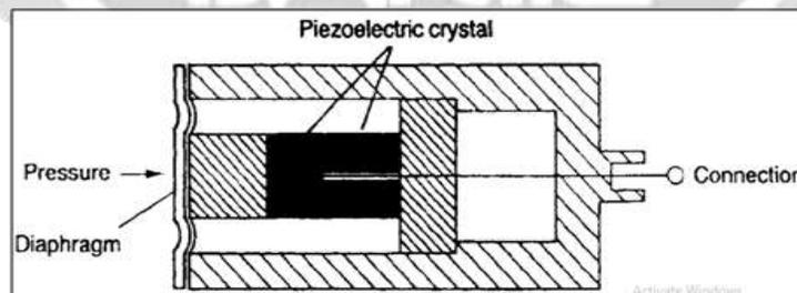
**Fig. 3.2** Electrical amplifiers are connected to a piezoelectric crystal.
