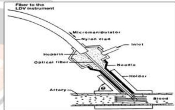
**Fig. 7.2** special probes for measurement of blood velocity.
