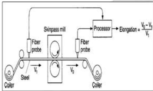
**Fig. 7.1** Fiber-optic laser Doppler velocimeter at a rolling mill controls pressure by measuring input speeds.
