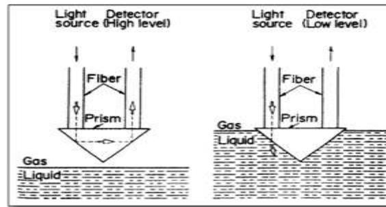
**Fig. 6.5** Principle of operation of a liquid level sensor with a prism attached to two optical fibers.
