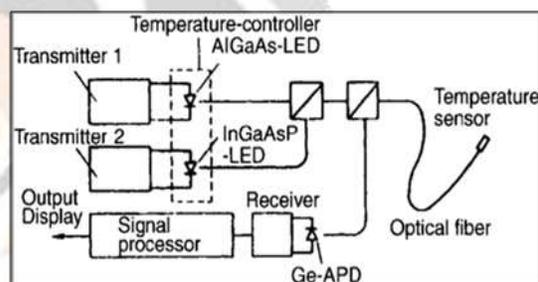
**Fig. 2.3** System configuration of the optical-fiber thermometer with GaAs light absorber.
