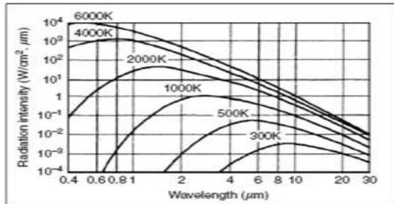
**Fig. 2.7** Spectral distribution of blackbody radiation.
