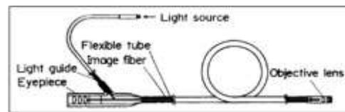
**Fig. 10.2** Basic structure of fiber scope.
