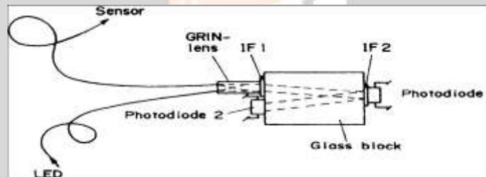
**Fig. 2.6** Optical system of optical-fiber thermometer based on temperature-dependent photoluminescence.
