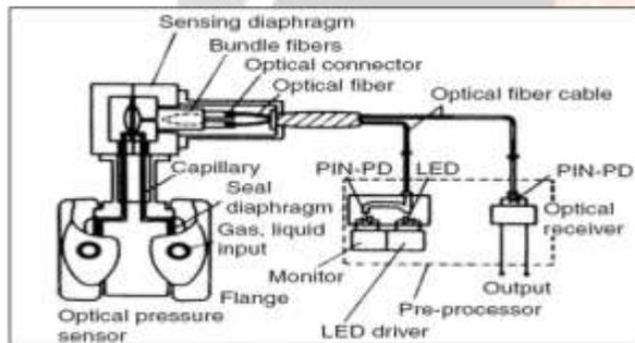
**Fig. 4.1** Schematic diagram of a fiber-optic pressure sensor using Y-guide probe with a diaphragm attached.
