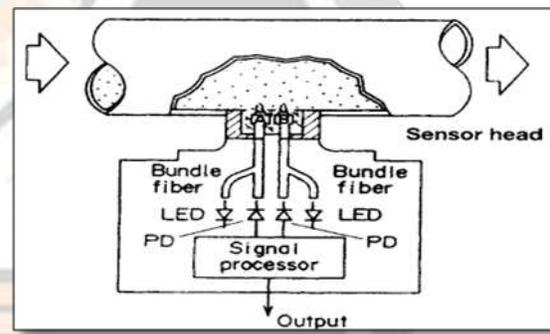
Fig. 6.4 Flow sensor using two Y-guided probes based on a correlation technique.
