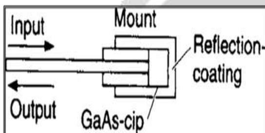
**Fig. 2.2** Sensing element of the optical-fiber thermometer with GaAs light absorber
