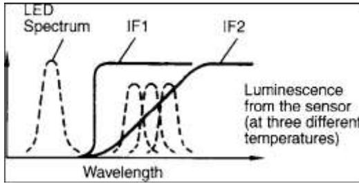
**Fig. 2.4** Operating principle of optical-fiber thermometer based on temperature-dependent photoluminescence from a GaAs epitaxial film.
