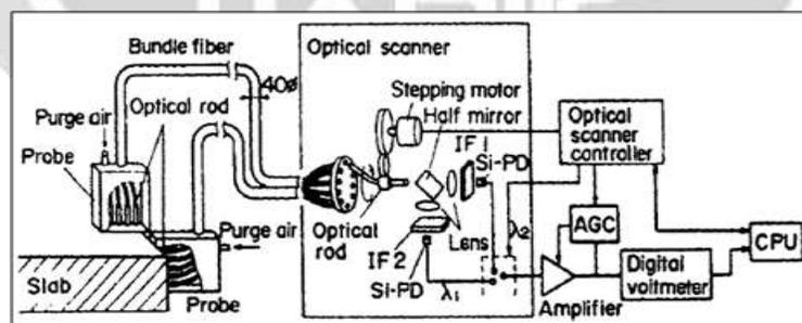
**Fig. 2.9** Temperature distribution measurement of steel slabs by an optical-fiber pyrometer using two-wavelength method.
