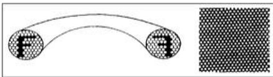
**Fig. 10.1** Image transmission through an image fiber.
