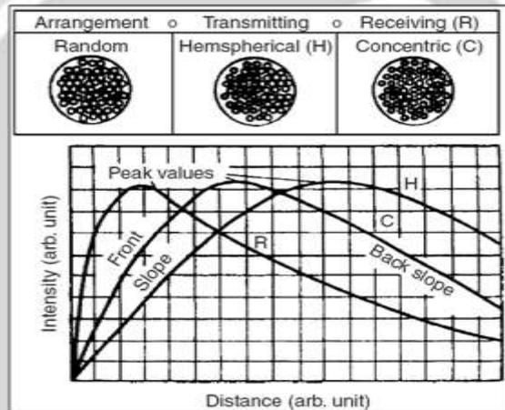
**Fig. 5.2** Relative intensity of returned light for three fiber optic arrangements.
