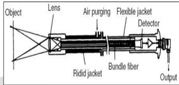
**Fig. 2.8** Schematic diagram of an optical-fiber pyrometer.
