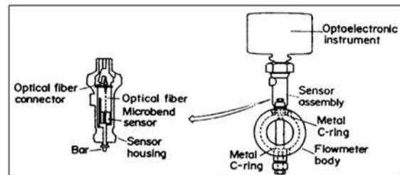
**Fig. 6.2** Schematic diagram of a vortex-shedding flow sensor
