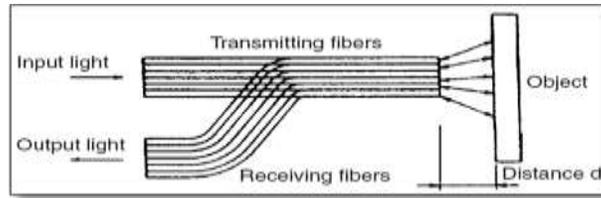
**Fig. 5.1** Principle of operation of fiber-optic mechanical sensor using a Y-guide probe.
