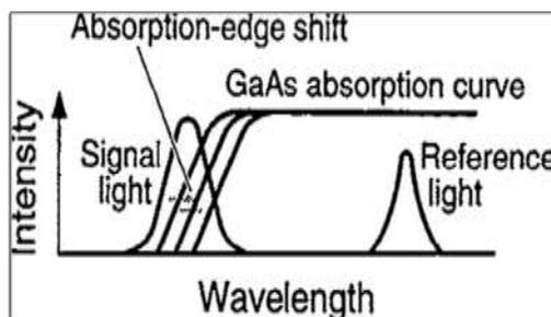
**Fig. 2.1** Operating principle of optical-fiber thermometer based on temperature-dependent GaAs light absorption.
