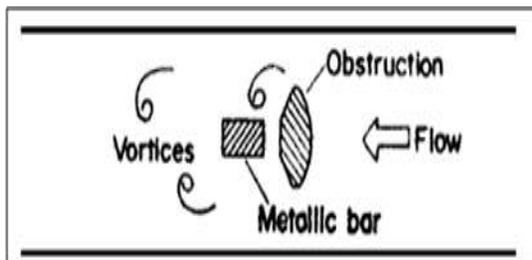
**Fig. 6.1** Principle of operation of a vortex-shedding flow sensor.
