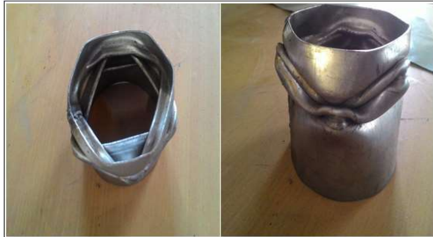
Fig -5: Circular Crash Box after Impact test
