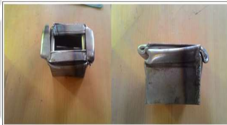
Fig -3: Square Crash Box after Impact test
