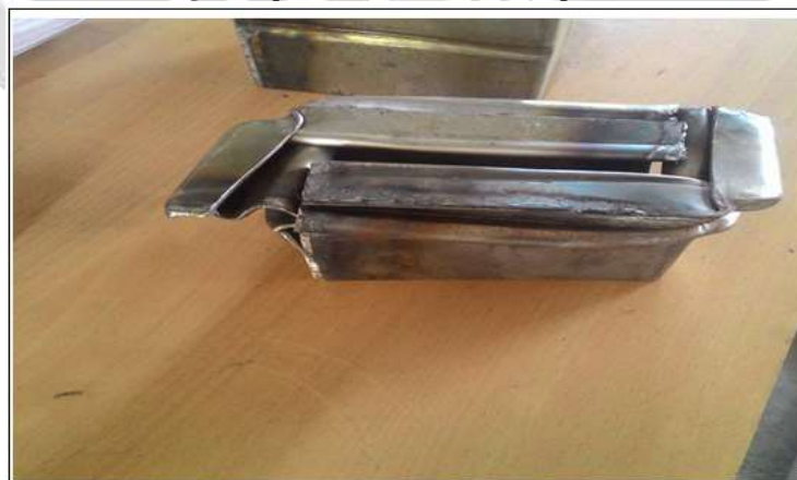
Fig -4: Rectangular Crash Box after Impact test
