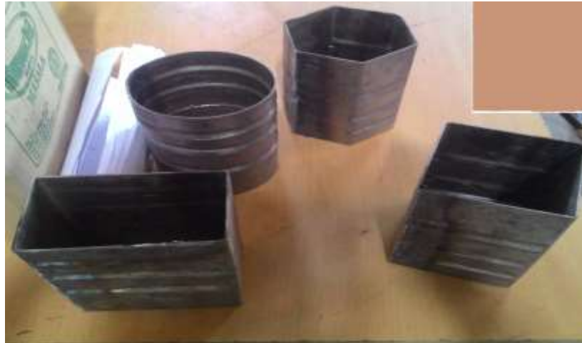
Fig -2: Different Shapes of Crash Box before Impact test
