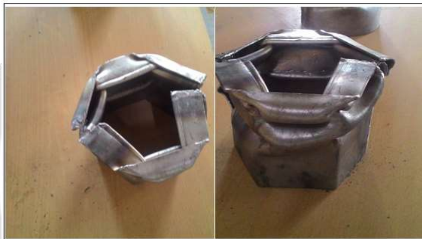
Fig -6: Hexagonal Crash Box after Impact test
