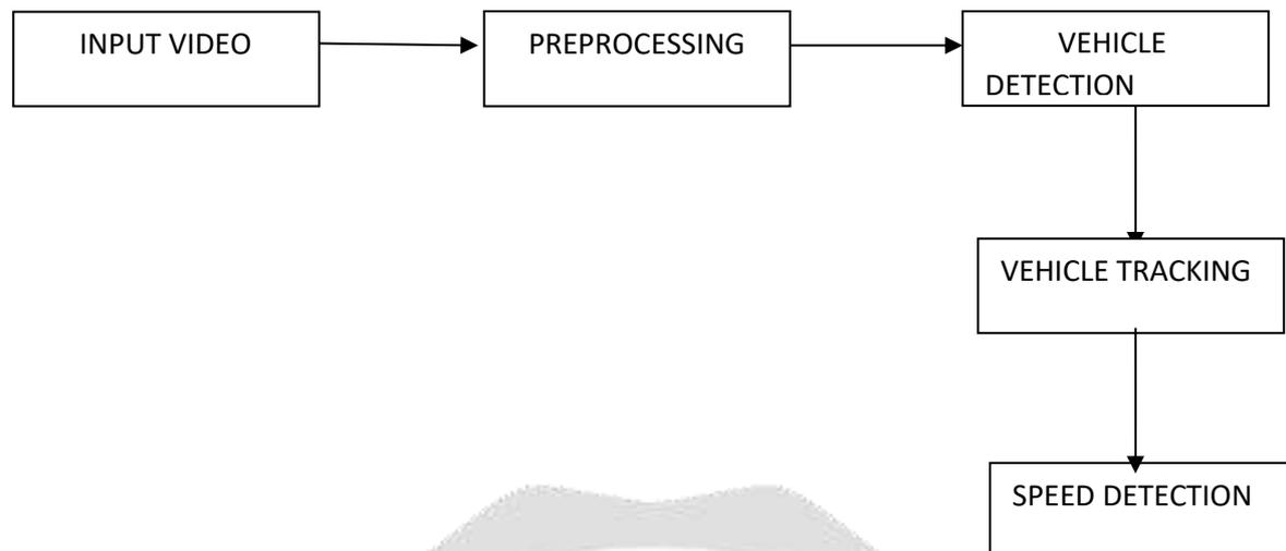
Fig. 1: Block diagram of vehicle speed detection system
