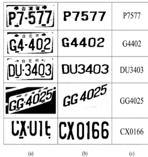
Fig -3: Example of license number identification (a) Locating license plate (b) Region Segmentation (c) Licence number identification.
