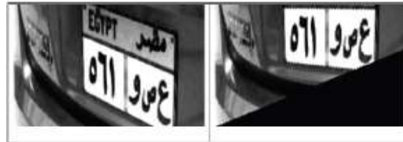
Fig -4: (a) the original image after skew; (b) after applying the de-skew (shear) operation using Hough transform, It is clear that the plate became axes
