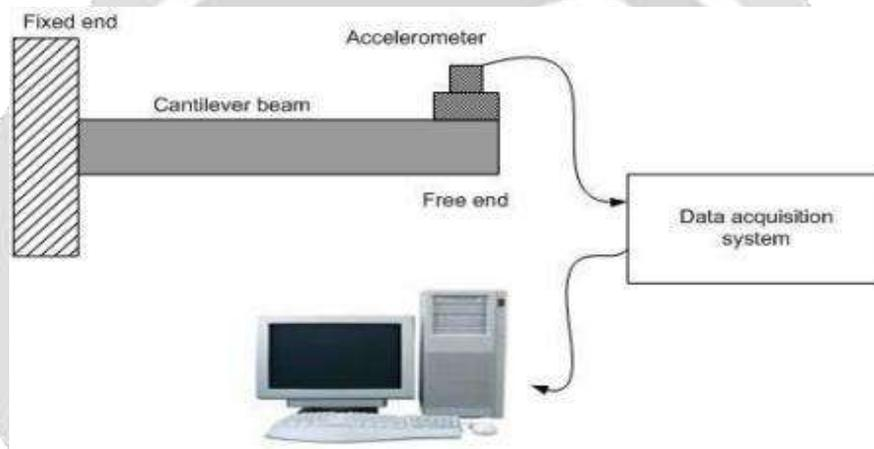
**Fig. 2.1:** An experimental setup for the free vibration of a cantilever beam
