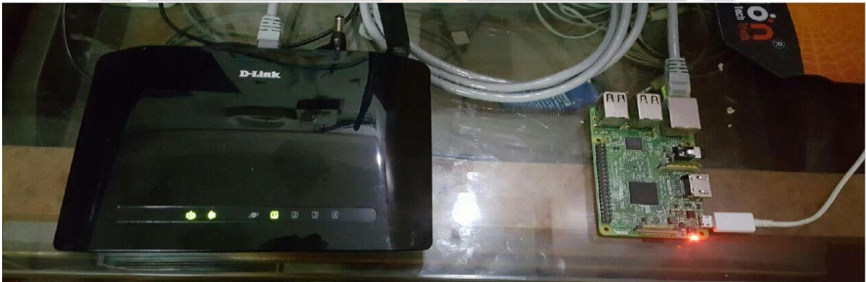
Fig 3.2.1: Raspberry pi is connected to router with the help of Ethernet cable
