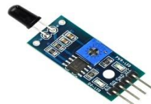
Fig -4 Fire Sensor
