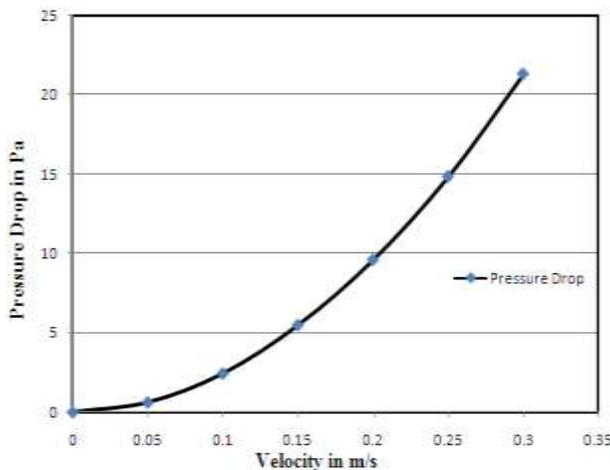
Fig-3 Pressure Drop versus Velocity
