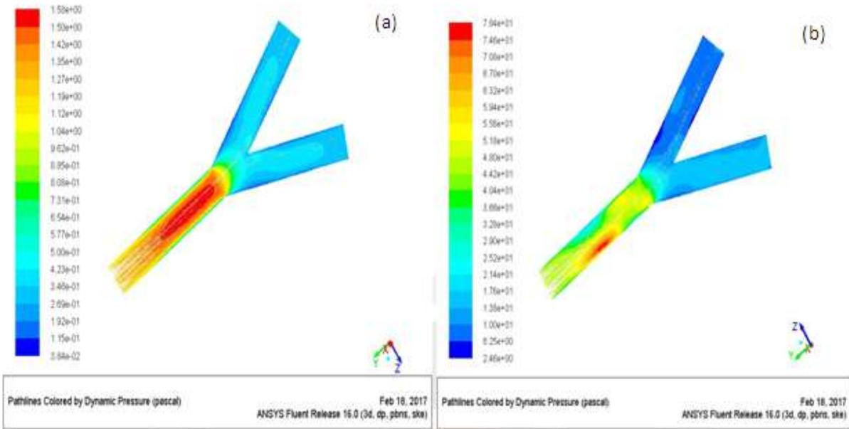
**Fig-8.a** Pressure Distribution for Velocity of 0.05 m/s
