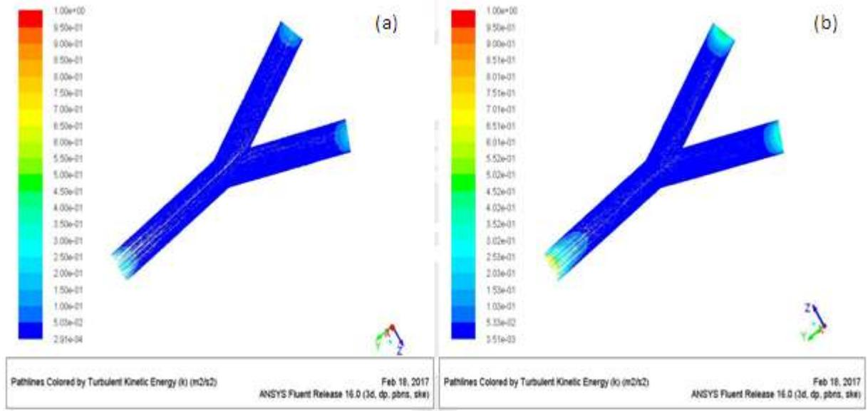
**Fig-9.a** Turbulence Existence for Velocity of 0.05 m/s
