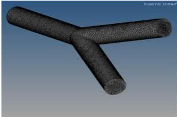
Fig-2.a. Meshed Model of Y-duct
