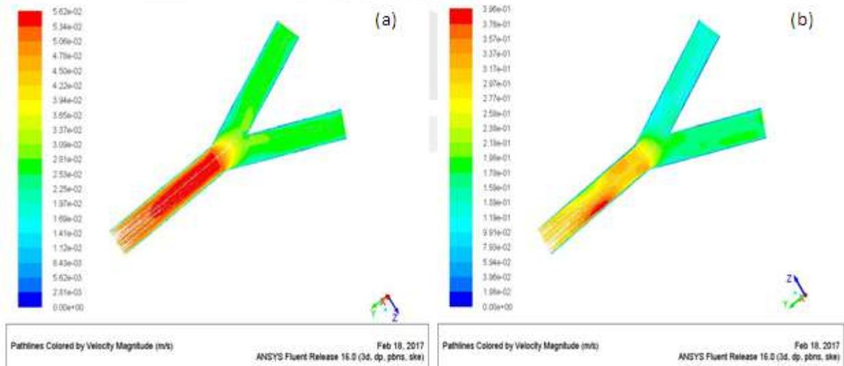
Fig-7.a Velocity Distribution having the rate of 0.05 m/s
