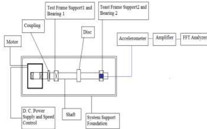
**Fig. 4.** Experimental arrangement
