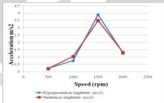
**Fig. 9** Numerical and experimental acceleration values compression at different speed with 0.5 kg disc for 45° crack at 100mm.
