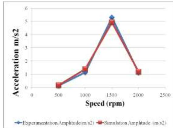
**Fig. 8** Numerical and experimental acceleration values compression at different speed with 0.5 kg disc for healthy shaft
