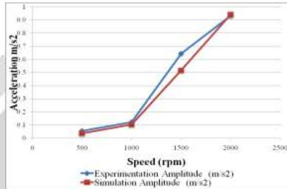
**Fig. 10** Numerical & experimental acceleration values compression at different speed with 0.5 kg disc for 60° crack at 100mm.
