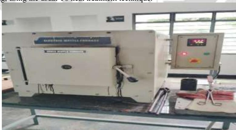
**Fig: Solution Heat Treatment using muffle furnace**
