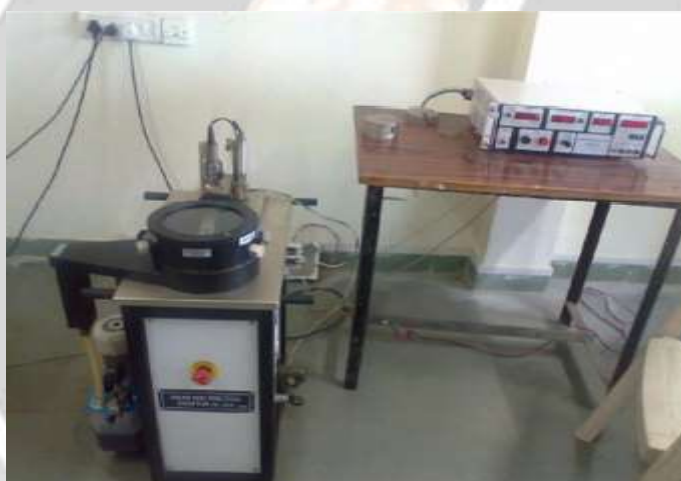
Figure-1: Set-up of pin-on-disc Tribometer (TR-20LE)
