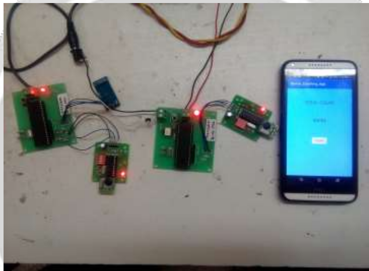
Fig.3 - Wireless Monitoring For Machine Part Counter
