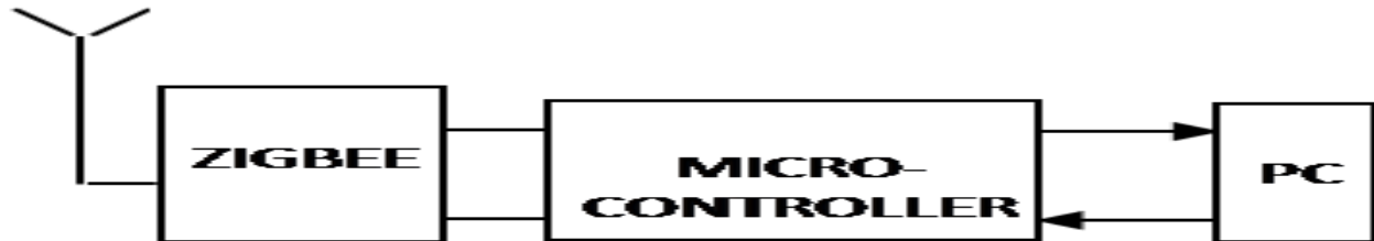
Fig.2: Base Station Gateway
