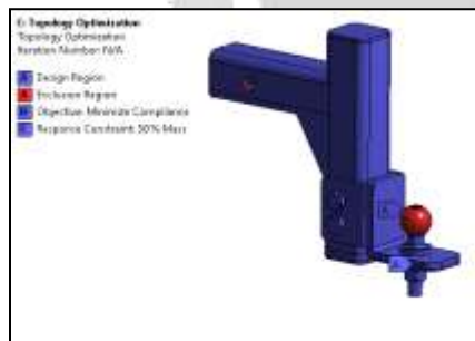
Fig. 11 Details of boundary conditions for topology optimization
