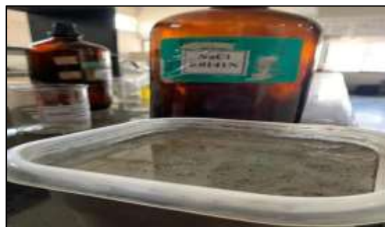
Fig-1: Putting chlorides on top of it when hardened
