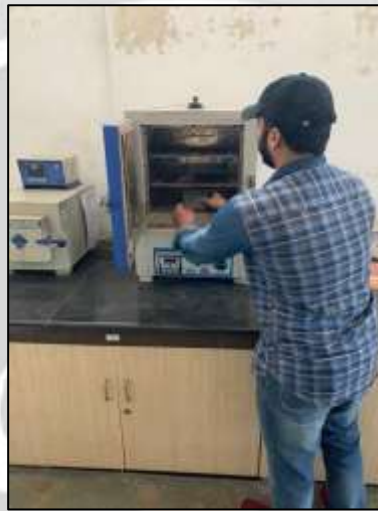
Fig-2: Placing following cube in oven for fast diffusion of chlorine
