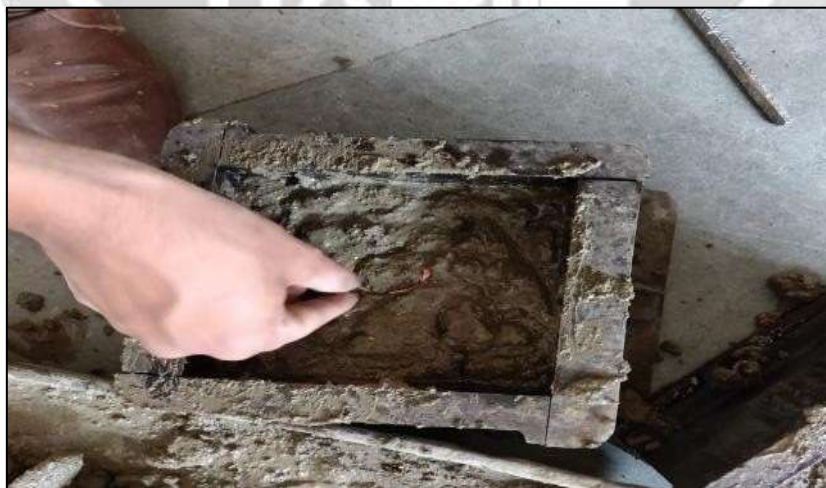
Fig-3: Casting Cubes and providing sensors
