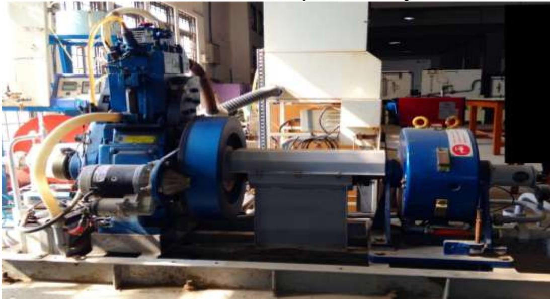
**Fig 3.4 Photographic view of single cylinder four stroke petrol engine**
