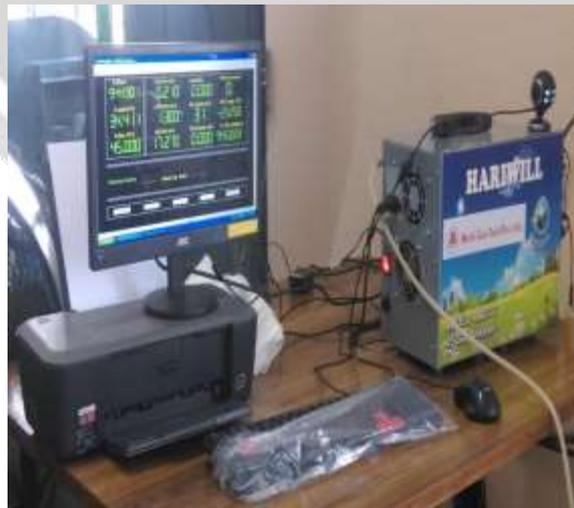
**Fig 3.5 Exhaust Gas Analyser**
