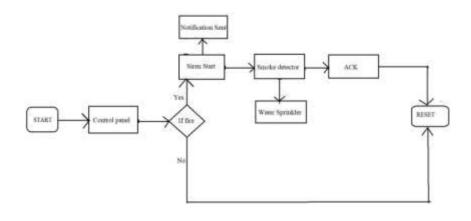
Fig: 3.1 Fire alarm system flowchart operation
