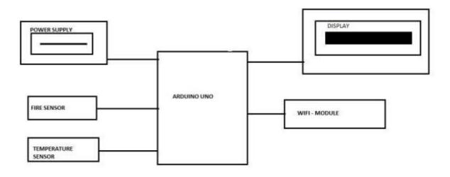
Fig 2.1 Architecture of Fire alarm system
