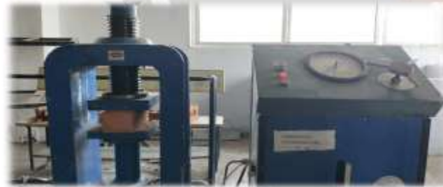
Figure No-2: Set-up of Compressive Strength Test
