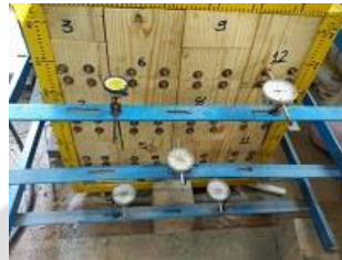
Fig- 8 Location of mechanical dial gauges on the facing panel
