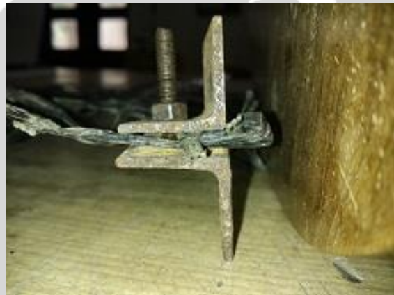
Fig- 4 Mechanical connection of geo-grid with steel clamps
