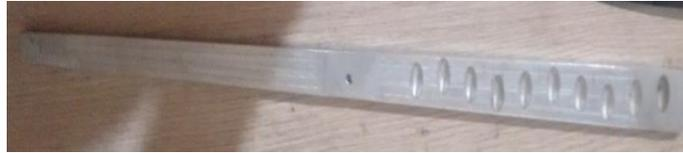
**Fig No. 13** Divergent plate with Offset arranged Elliptical dimple geometry
