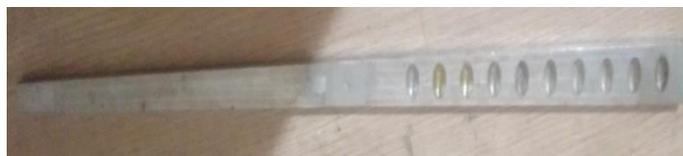
**Fig No. 12** Divergent plate with Inline arranged Elliptical dimple geometry
