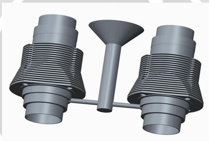
Figure 8 : 3D model of Gating System
