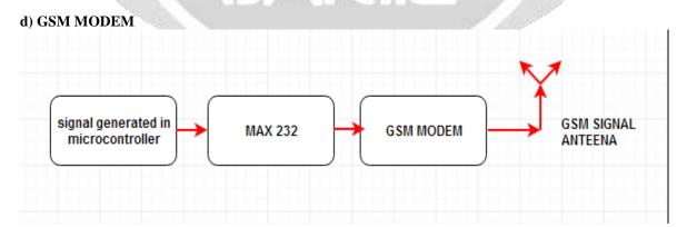
The figure shows the wireless GSM receiver set up at the receiver end. Here we are using GSM SIM900 within built GPRS. The signals are transmitted through GPRS which is received through SMS.
