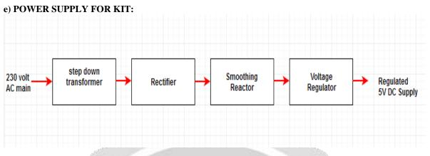
In the above block diagram we can see that power supply required for kit here firstly 230 volt AC main supply step down into the about 9 volt AC then this again converted into 5 volt and further 5 volt AC is converted into DC supply then we use smoothing reactor for smoothing purpose then using voltage regulator ic we can get 5 volt pure DC supply which is required for kit.
