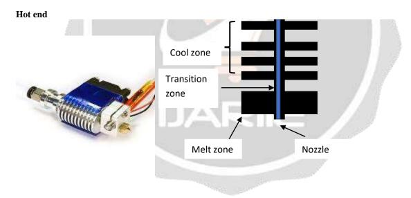
The hot end is the most important part of a 3d printer. the filament passed through the extruder comes to the hot end where there are four parts cooling zone, transition zone, melt zone, and nozzle then in the melt zone, it melts at a specific melting temperature and comes out from the nozzle and prints the object on a heated bed.
