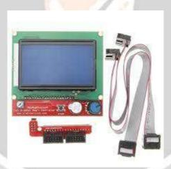
Lcd stands for liquid crystal display. The LCD is used to control the working of the 3d printer. It is connected to the Arduino with the wires, so the coding for the 3d object in the Arduino is directly run with the use of an LCD.
