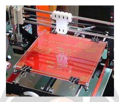
A heated bed is another most important part of a 3d printer. The objects are printed on this heated bed. on this heated bed there is a glass bed or a metal bed also so that we can remove the printed object easily. Heat beds prevent issues like poor adhesion to print bed, poor adhesion between layers, thermal runaway, and warping. the result of using a heated bed can be greater precision and less waste, due to the prevention of early or uneven cooling
