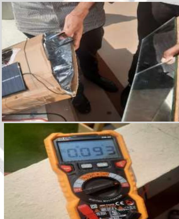
Fig-9: Bottom Solar panel with light reflector arrangement and its measurements.
