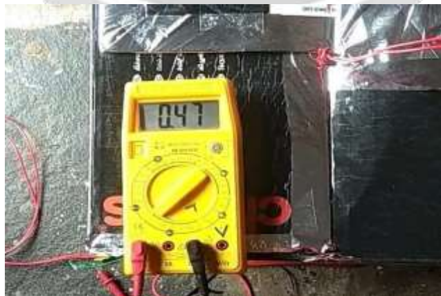
Fig-10: Solar panel with aluminum & mirror light reflector arrangement and its measurements.
