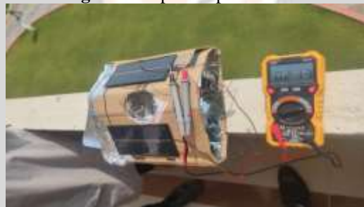
Fig-5: Top Solar panel Measurement without Light Reflector
