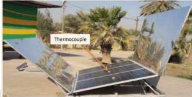
Fig-1: Schematic View of Solar panel with Light Reflector Arrangement
