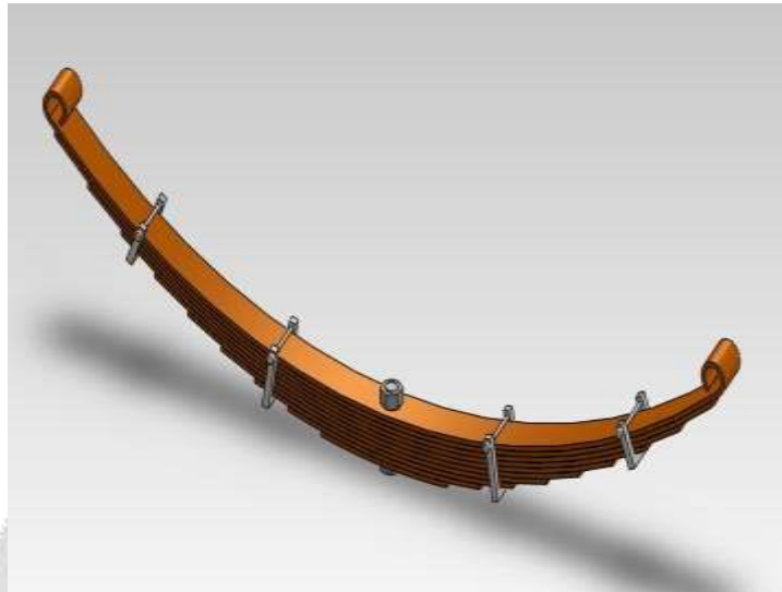
Fig 1 Solid model of steel leaf spring created in Solid Work 2011 and imported it's for analysis in ANSYS
