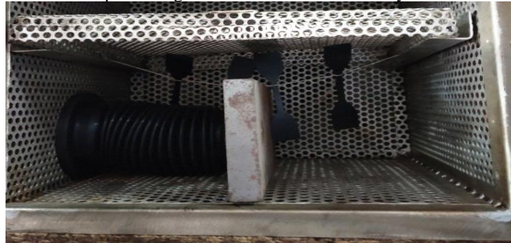
Fig. 5.2: Hot air aging Test setup
