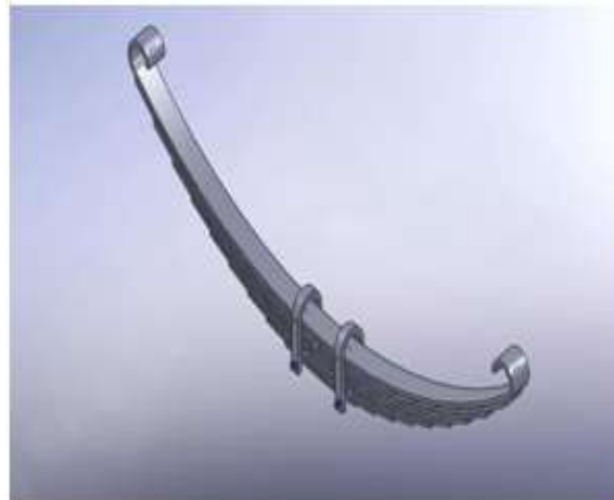
Figure 1. Isometric view of existing leaf spring
